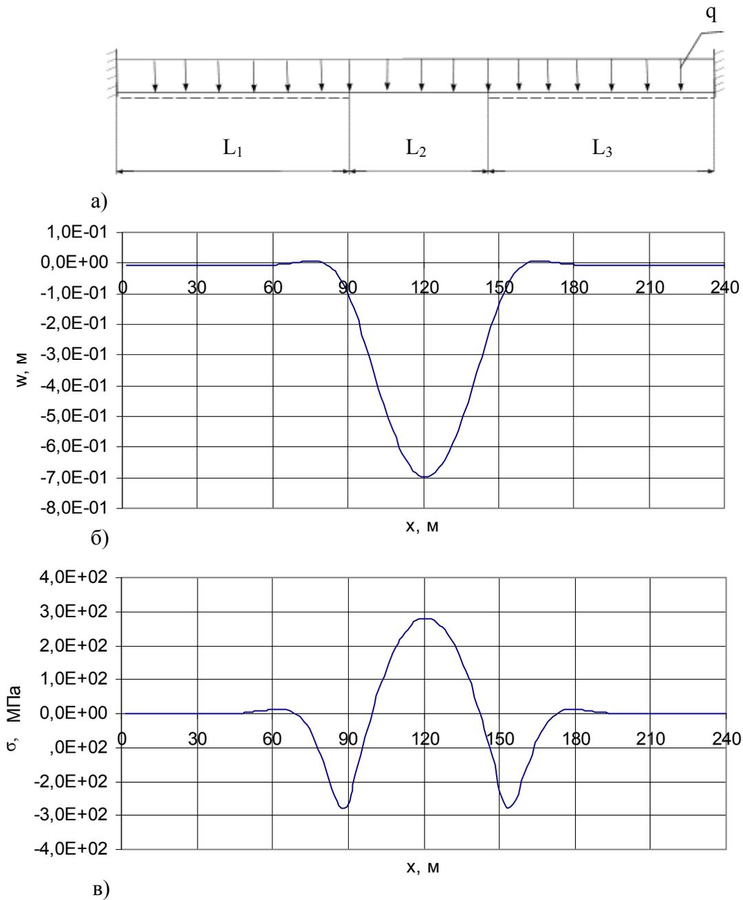
Fig.2 The calculation of main parameters of SDC of the submerged pipeline in the carst zone: a) a designed pipeline diagram ( $L_1=L_3=90\text{m}$ ,  $L_2=60\text{m}$ ;  $p_0=0$ ;  $\Delta t=50\text{ deg.C}$ ); b) diagram of saggings; c) bending stresses
