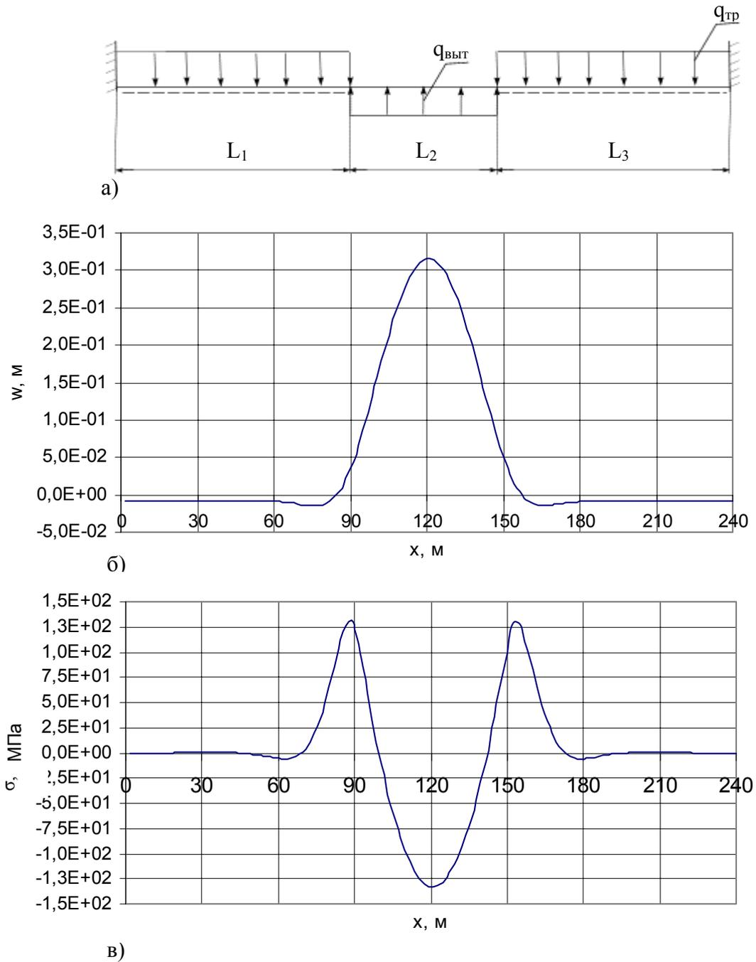
Fig.4 The calculation of main parameters of SDC of the submerged pipeline in the carst zone: a) designed pipeline diagram ( $L_1=L_3=90\text{m}$ ,  $L_2=60\text{m}$ ;  $p_0=0$ ;  $\Delta t=50 \text{ deg.C}$ ); b) diagram of saggings; c) bending stresses
