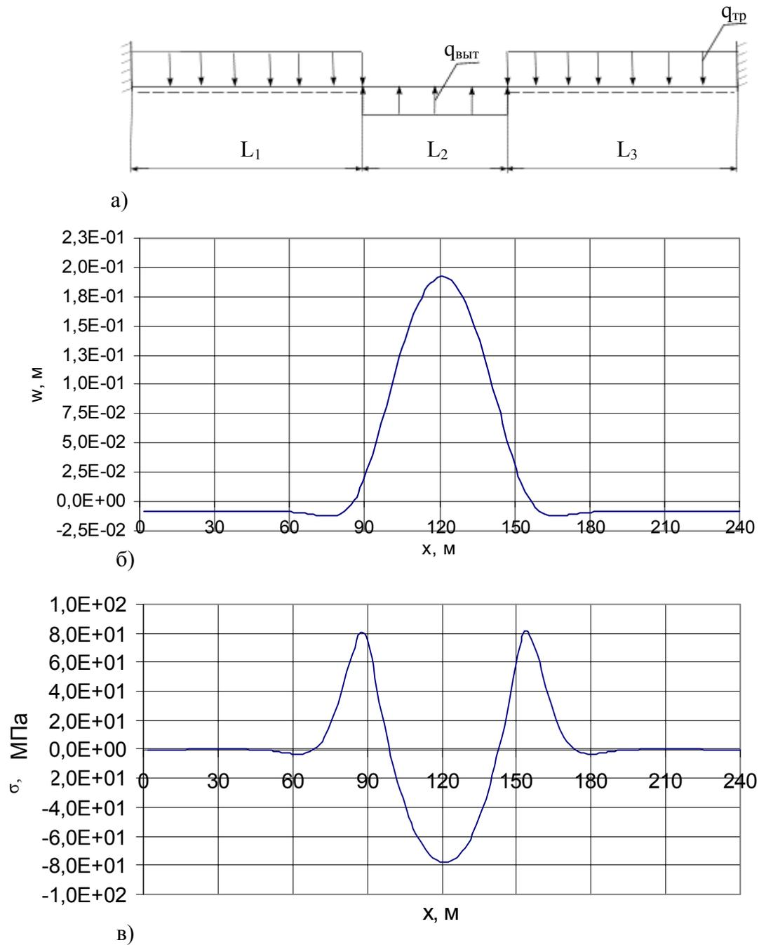
Fig.3 The calculation of main parameters of SDC of the submerged pipeline in the carst zone: a) designed pipeline diagram ( $L_3=90\text{m}$ ,  $L_2=60\text{m}$ ;  $p_0=7,5\text{Mpa}$ ;  $\Delta t=20\text{ deg.C}$ ); b) diagram of saggings; c) bending stresses
