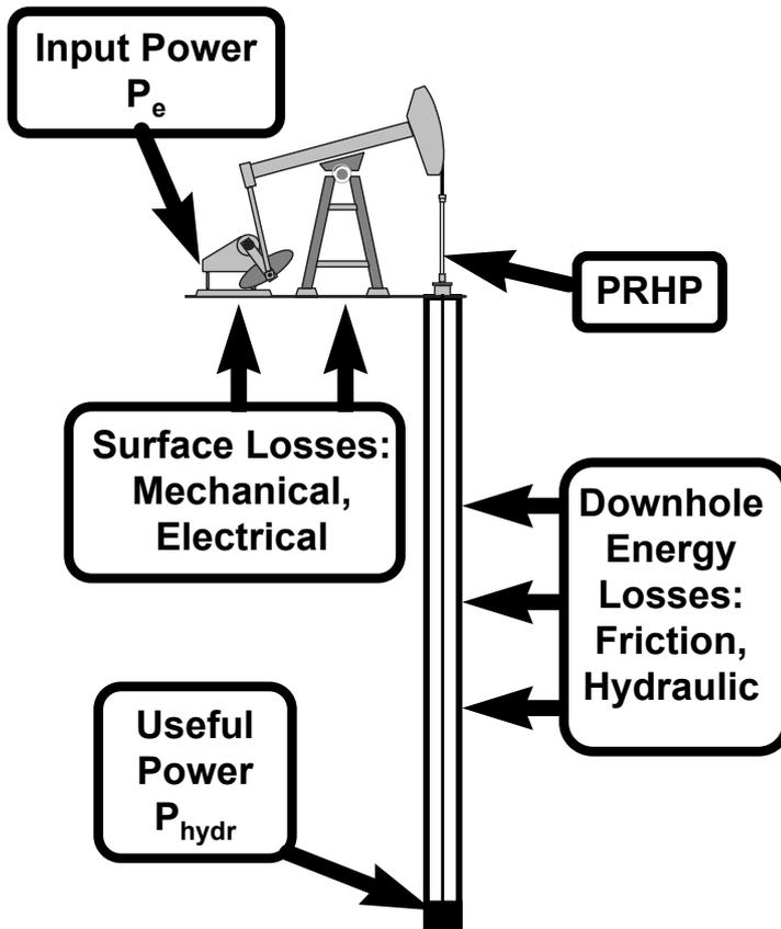
**Fig. 1. Energy flow in the sucker-rod pumping system**
