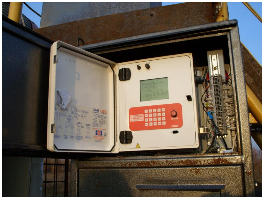
Figure 3. The control station of SRP with controller Lufkin Automation (USA)
