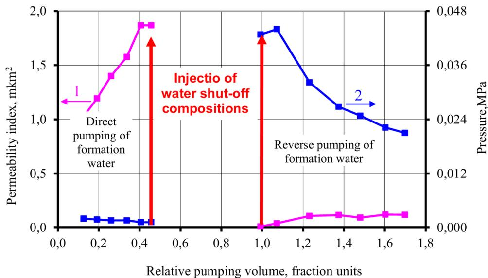
Fig. 3. Behavior of pumping pressure and permeability of water-saturated reservoir model after its treatment with 50 % water solution “OVP-1”:
