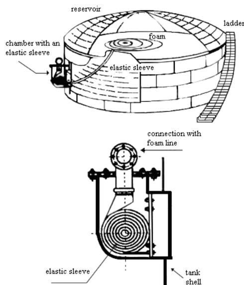
Fig. 1. Fire Extinguishing Systems for the foam supply in bottom of the tank through a flexible hose to the fuel surface
