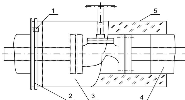
Fig. 1. Thermal isolation of reinforcement flange by insulating cylinder:
