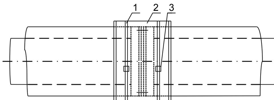
Fig. 1. Thermal isolation of flange coupling by heat-insulating cylinders:
