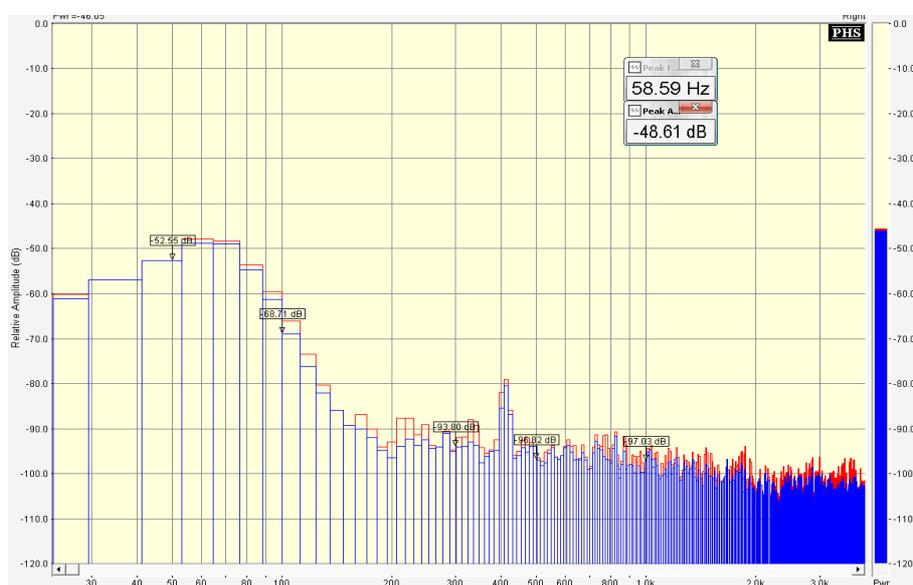
Fig. 2. The spectrum of the mechanical waves train at distance of 50 m from the point of shock formation in the program SpectraPLUS
