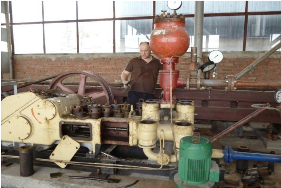
Figure 4. Dynamic test stand for valves
